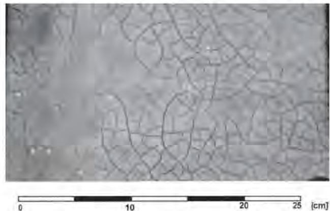
FIGURE 4.4 X-ray image showing desiccation cracks in the bottom layer of a GCL after 5 years in a landfill cover at Hamburg-Georgswerder. SOURCE: Melchior (2002).
