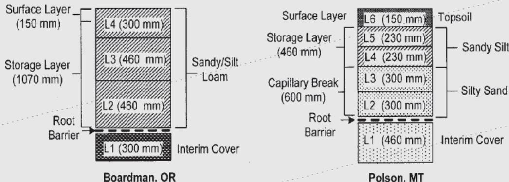
FIGURE 4.5 Schematic cross sections of alternative earthen final covers discussed in this case history. SOURCE: Ogorzalek (2005).
