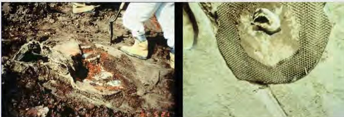
FIGURE 5.4 Damage to the primary liner. The hole extends through all of the geosynthetic layers into the top of the clay liner. SOURCE: Golder Associates, Inc.
