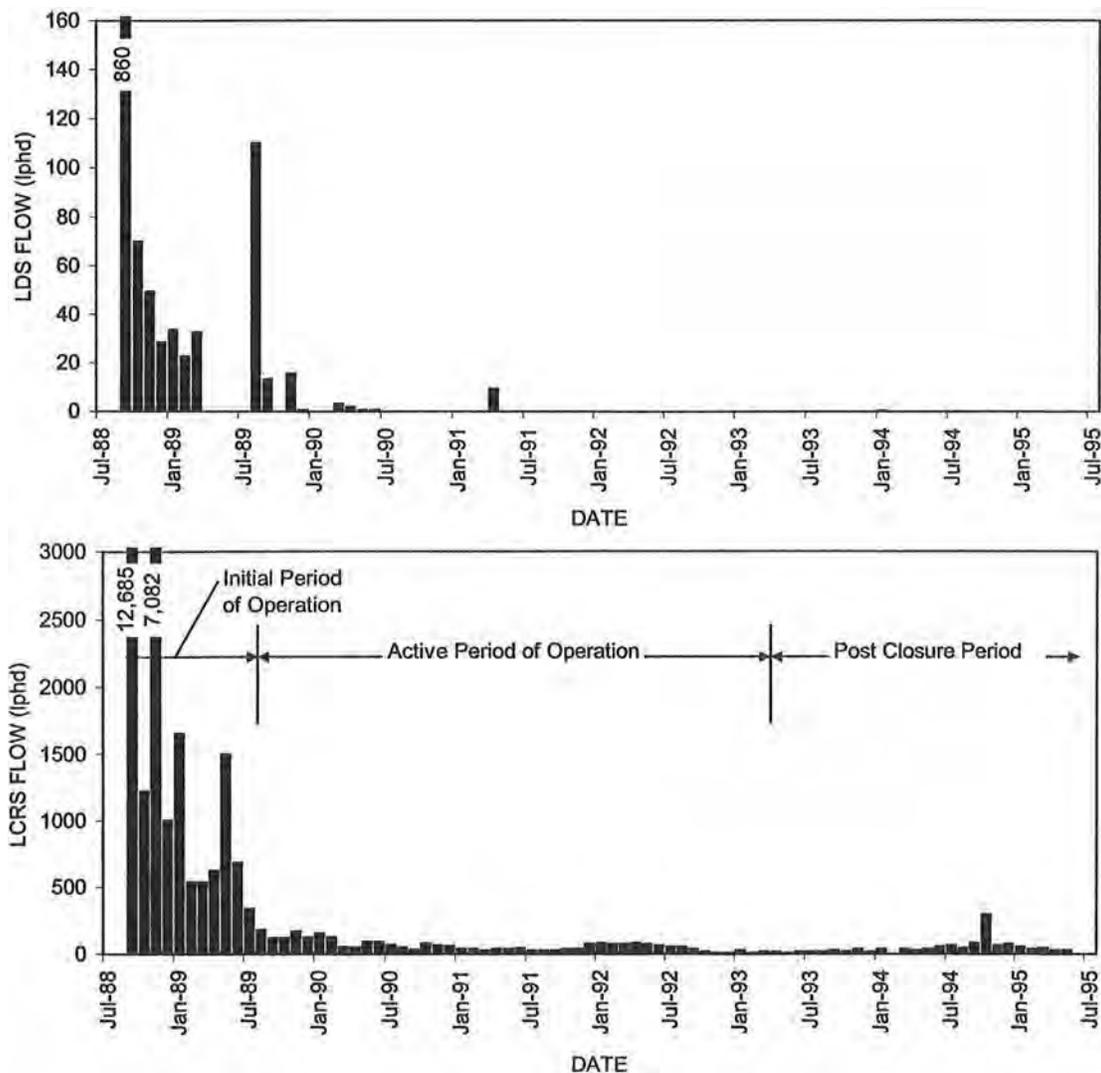
FIGURE 5.2 Leachate collection and removal system (*top*) and leak detection system (*bottom*) flow rates over time at an MSW landfill in Pennsylvania. SOURCE: Bonaparte et al. (2002).
